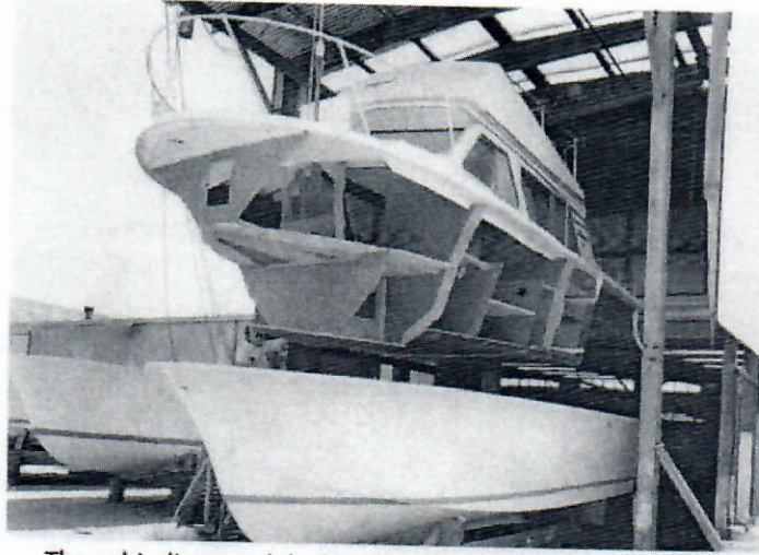
The cabin liner and deck are raised above a 26' Sedan hull.
