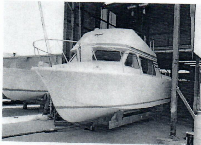
The cabin is fibreglassed to the hull.
